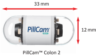
Figure 1.4: Representative commercial capsule endoscope (PillCam™ Colon 2) [21].
