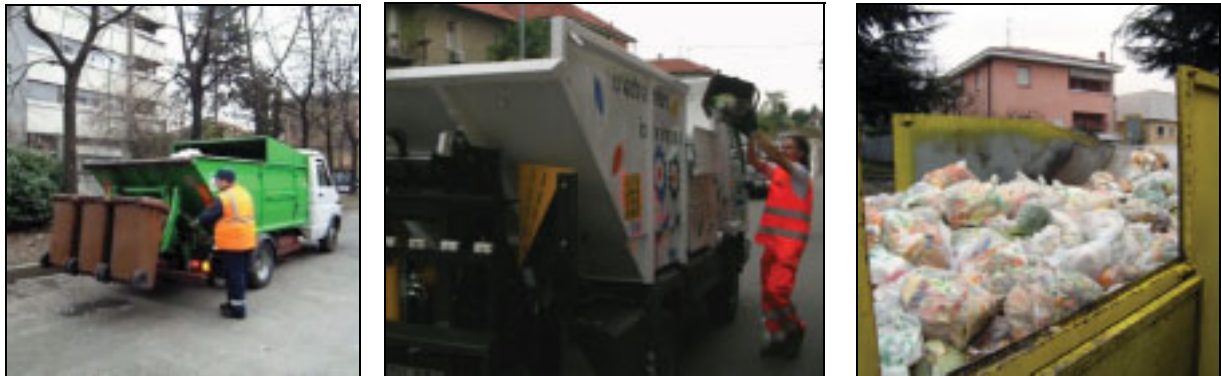
Figure 2 Mechanical and manual tipping of food waste in compostable bags
