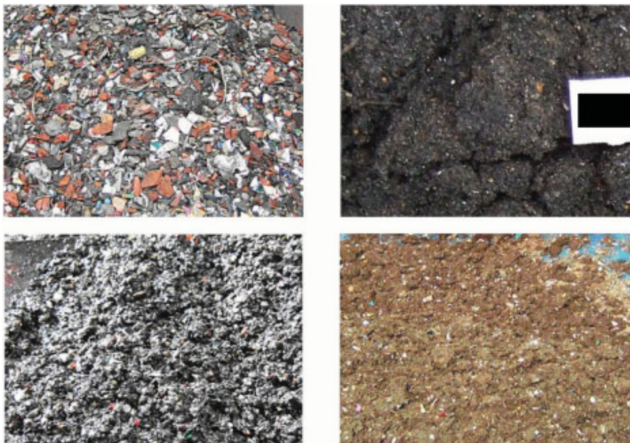
Figure 9: Various fractions from a biological and wet mechanical treatment step of an MBT
