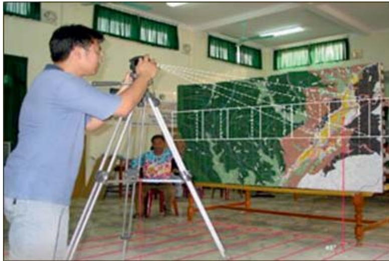
Figure 9. Capturing images with 60% overlap as indicated in white dotted line (Photo credits: Rambaldi, G., 2010).
