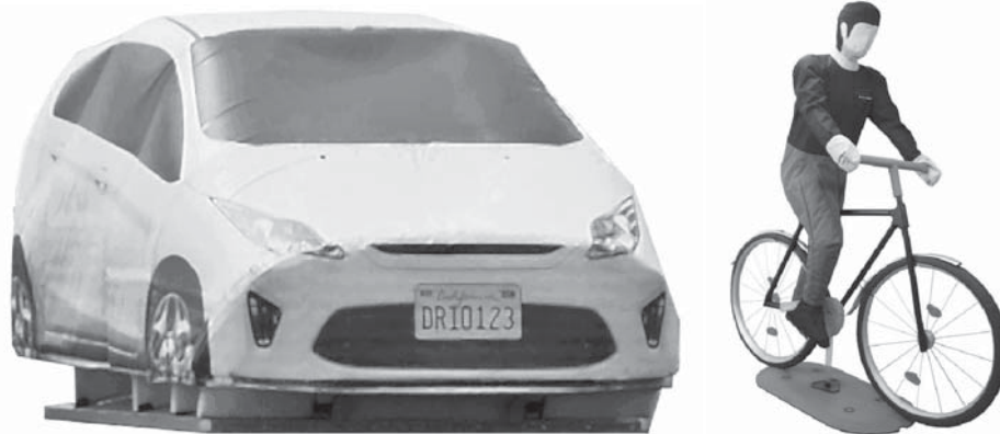
Figure 6: Testing advanced AEB systems in more complex traffic scenarios requires further advances in testing technology, such as 3D vehicle and cyclist targets
