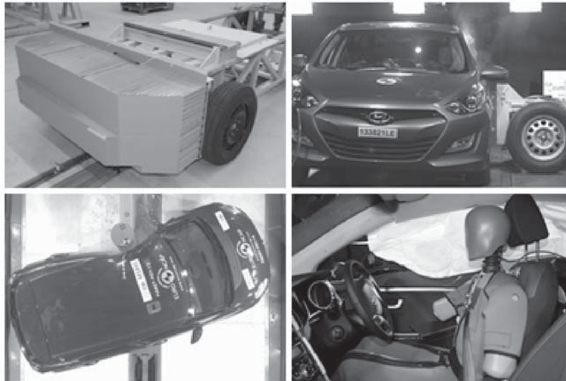
Figure 1: The updated Euro NCAP side impact crash tests using the Advanced European Mobile Deformable Barrier (AE-MDB) and the WorldSID mid-sized male dummy
