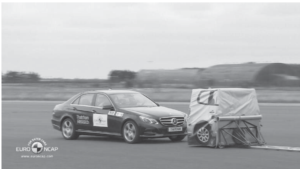
Figure 3: Euro NCAP started to assess AEB systems in 2014 using specially designed “impactable” vehicle target and test equipment
