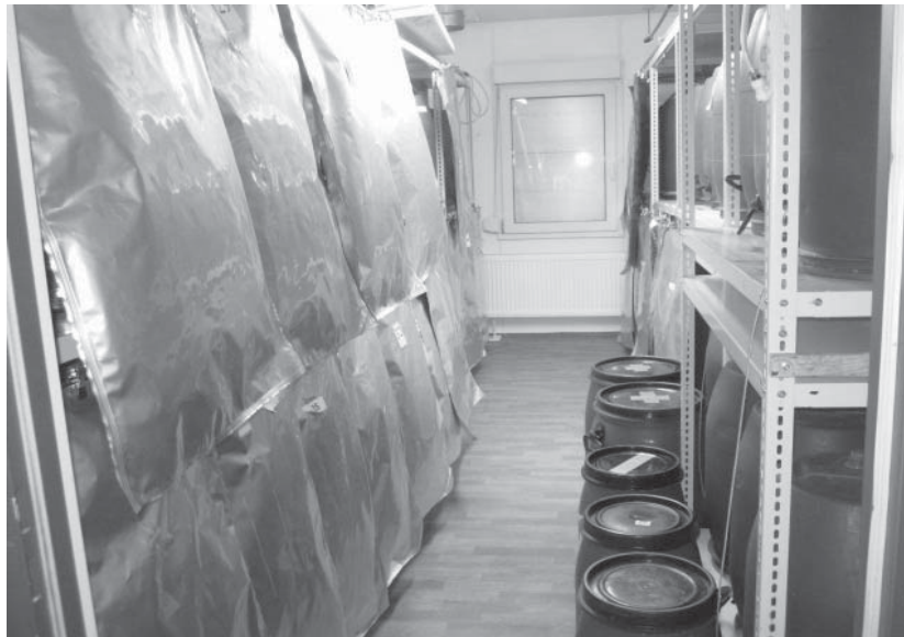
Figure 1 climatic chamber with barrels and gas bags during a biogas yield batch-test
