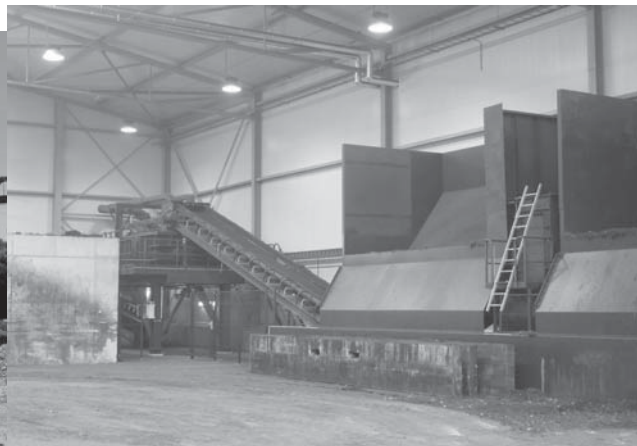
Picture 2: Mixer for structure material
