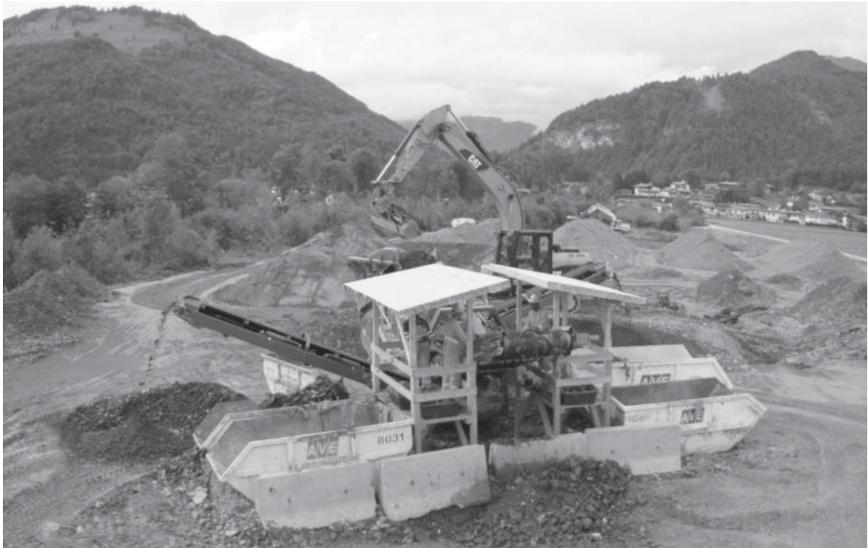
Figure 4 Core unit applied for dismantling the dump's inventory: a vibration screen producing a fine fraction (leaving the screen right hand side, windrows visible in background), a fraction 40 ... 70 mm (left) for further processing via air classifier, and > 70 mm out of which the fractions wood, glass, scrap metal and plastics/MSW are sorted manually.
