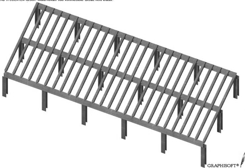
Figure 3-13: Axonometric view of key load bearing elements in variant 1
