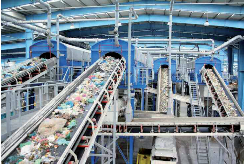
Figure 3: Drum screens to separate the MSW into five fractions after initial manual sorting and pre-shredding
