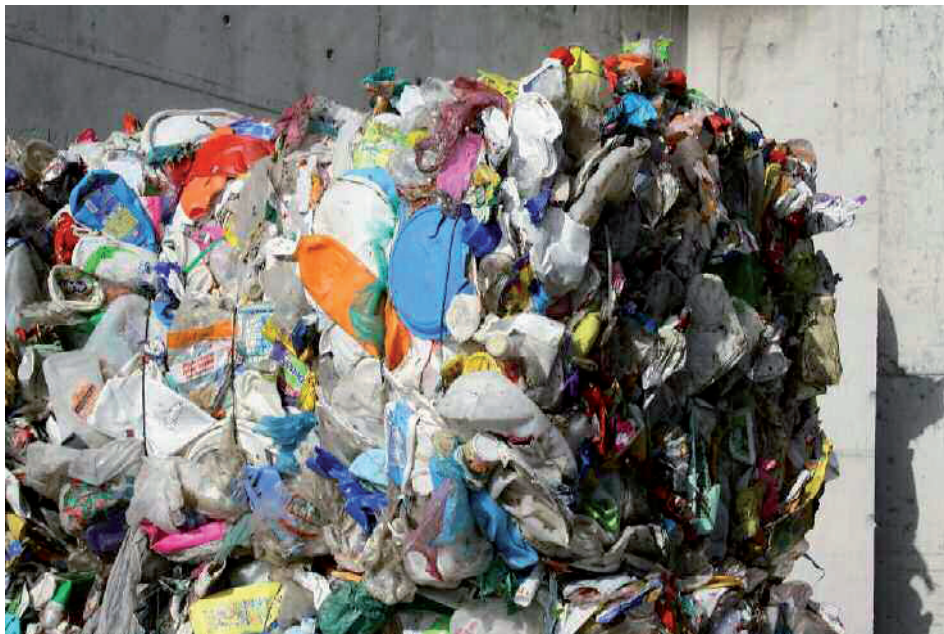
Figure 5: HDPE bale for recycling, gained from MSW treatment at the MBT Larnaka
