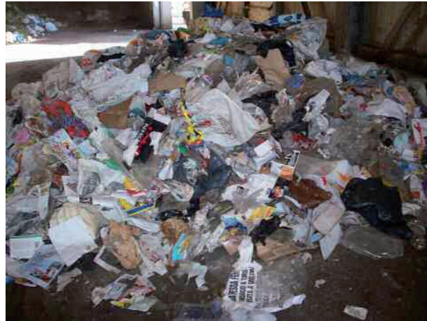
Figure 8 SRF separated by the aeraulic separator.
