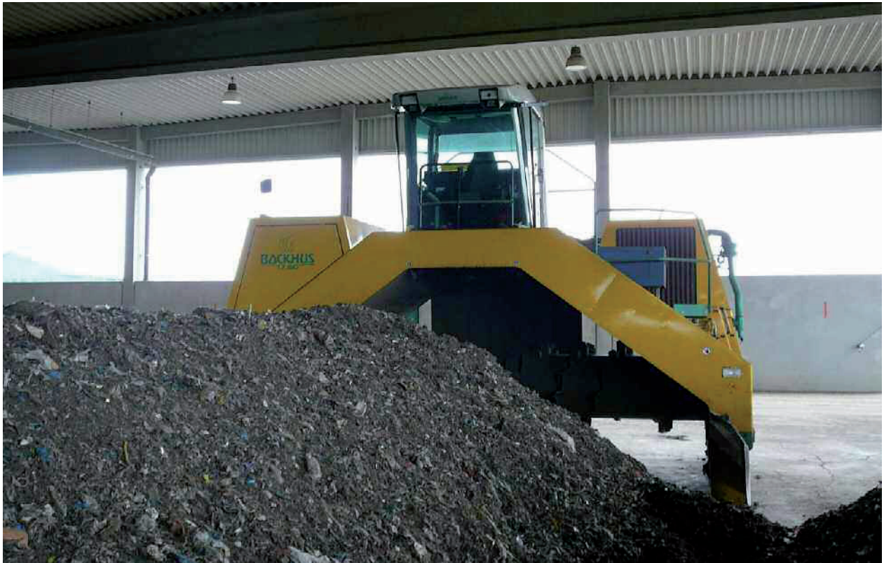
Figure 1 Self-propelled windrow turner BACKHUS 17.60
