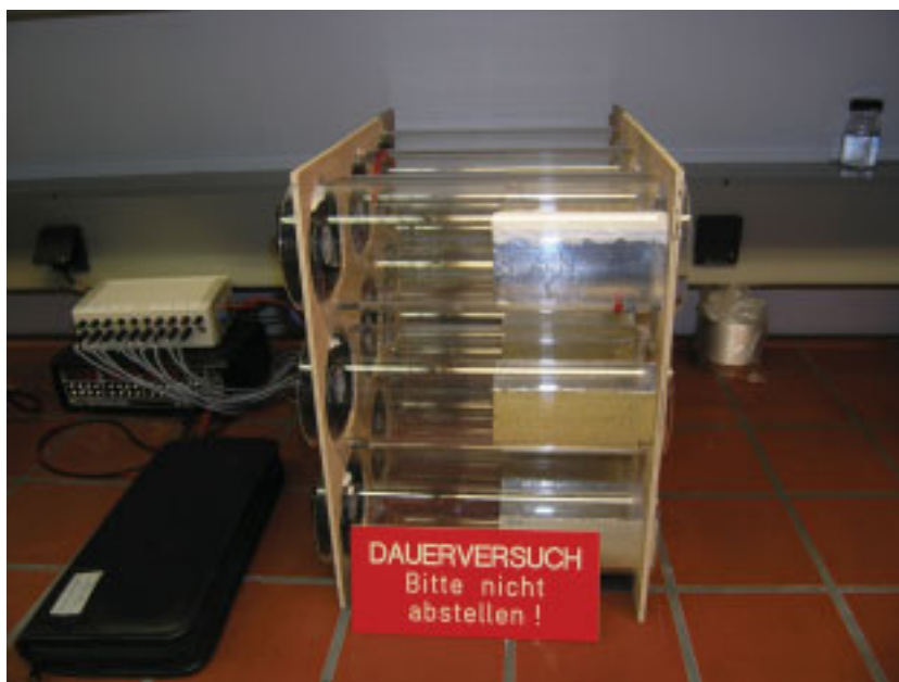
Figure 1: Set up built for the drying experiments at 23°C and 50% r.h.. The samples were placed in tubes where the air stream was maintained constant by means of small fans.
