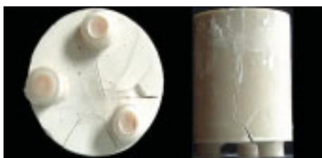
Figure 1: Crack development and propagation in hardened cement paste specimen
