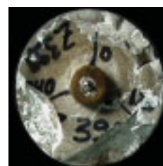
Figure 2: Specimen spalling related to crystallization pressure (cement paste)
