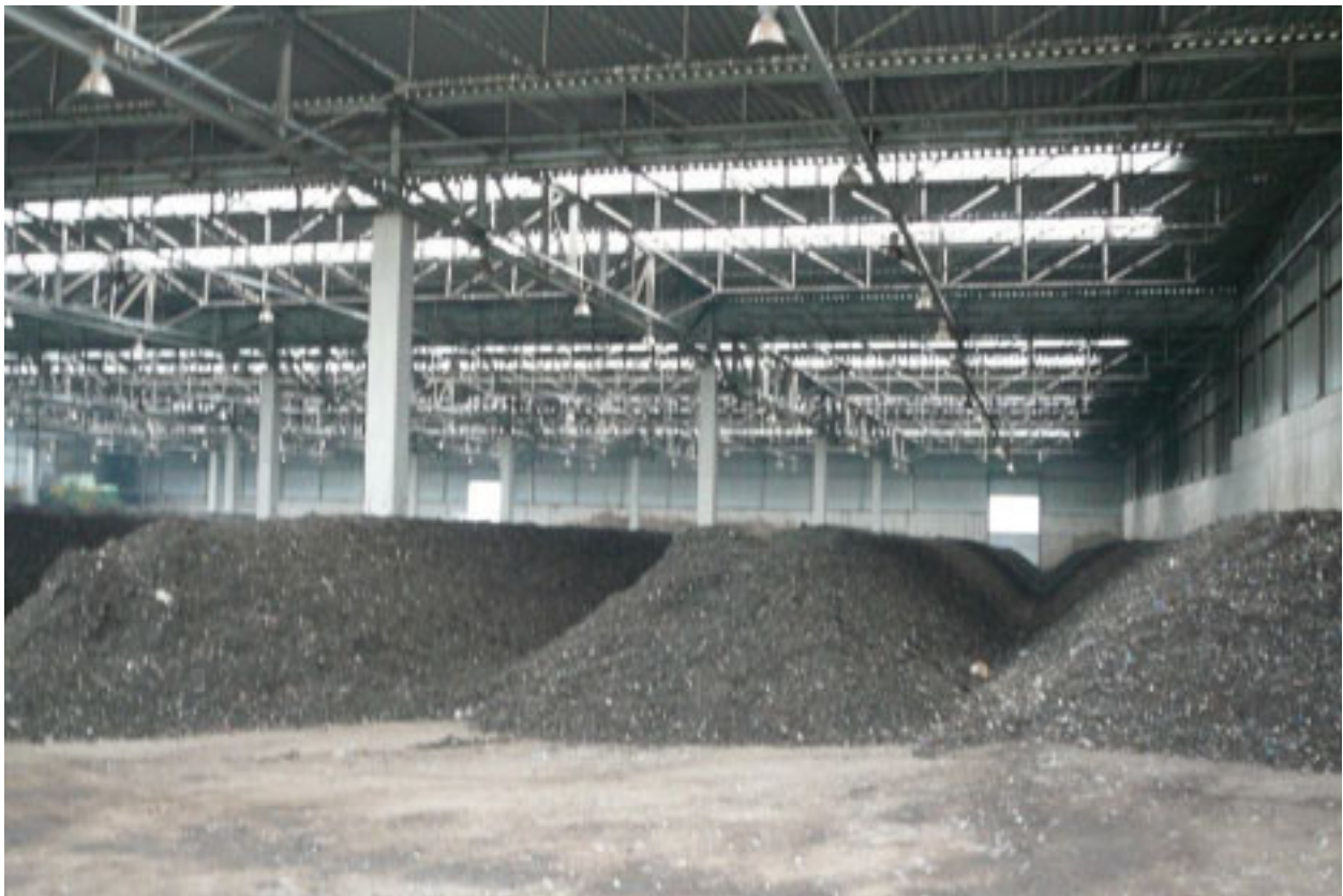
Figure 1: Maturation MBT Cröbern after changing to windrows
