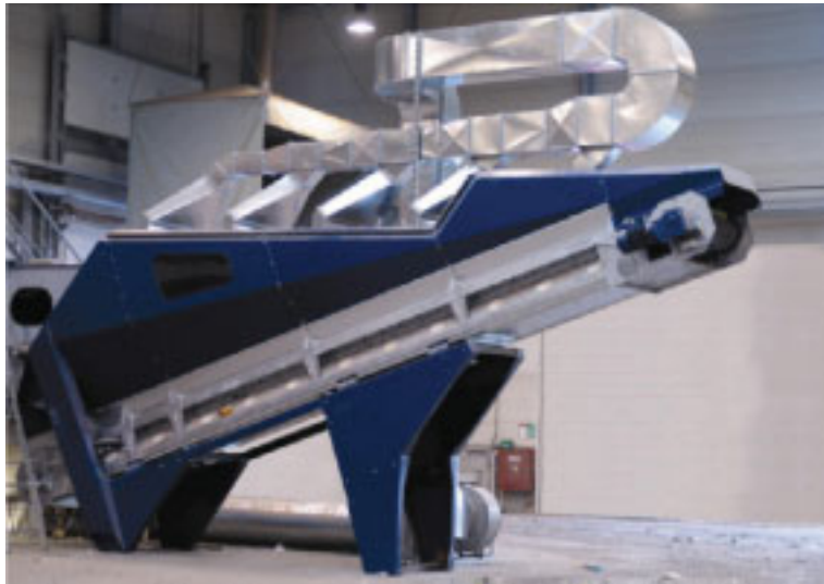
Picture 2: The awarded Lindner-Recyclingtech GmbH Heavy Fraction Separator HFS 1200
