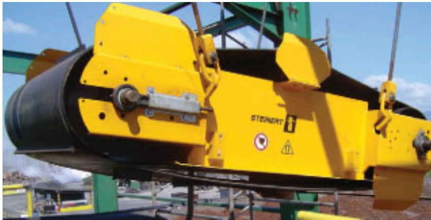
Figure 3: Suspended magnet positioned lengthwise above dropping point
