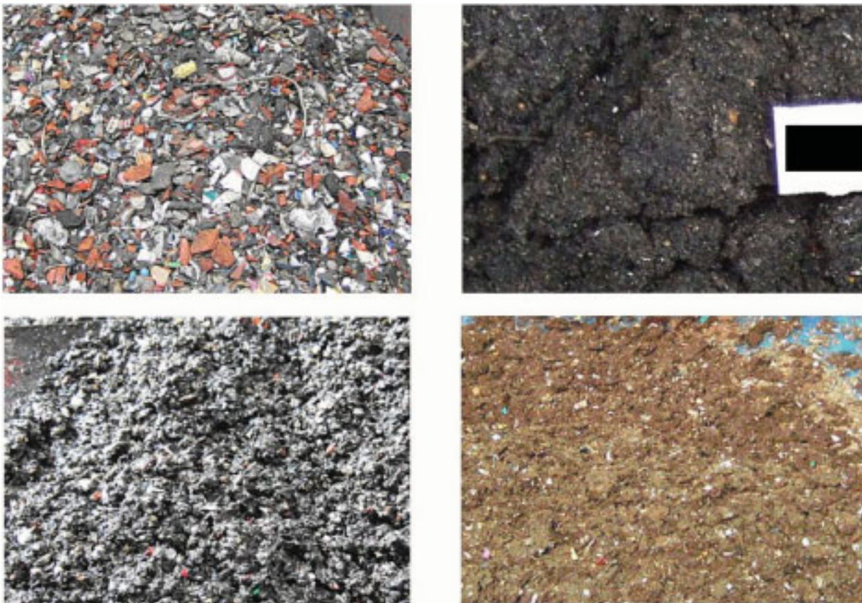
Figure 10: Various fractions from a biological and wet mechanical treatment step of an MBT
