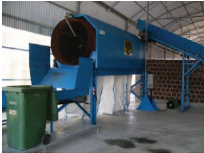
Figure 7 Rotating grate and sorting table
