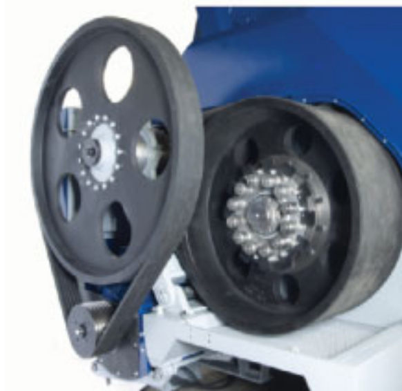
Picture 5: Innovative drive concept with centrifugal mass by Lindner-Recyclingtech GmbH
