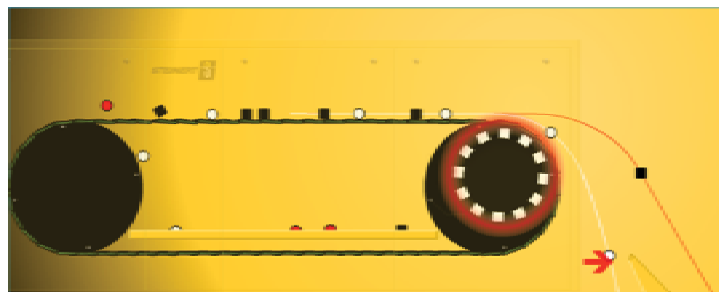
Figure 6: Eddy current separator with an eccentric pole system; adjustable; magnetic field only acts at the dropping point; red: iron particles can move freely
