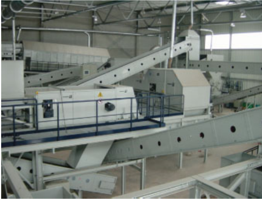
Figure 12: View of an RDF plant with an eddy current separator on the left and an induction sorting system combined with a near-infrared camera on the right side
